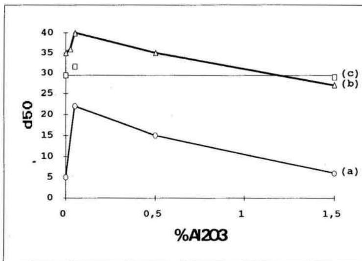
Figure 6. Aluminum effect on  $d_{50}$  of gypsum crystals: (a) "0" saturation (Rocha e Ciminelli, 1990) (b) 0,25 saturation (Leão e Ciminelli, 1992); (c) 0,87 saturation.
