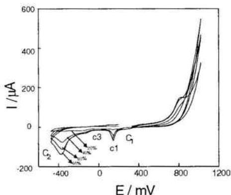
Fig. 3. Cyclic voltammograms of pyrite/pyrrhotite carbon paste electrode.
