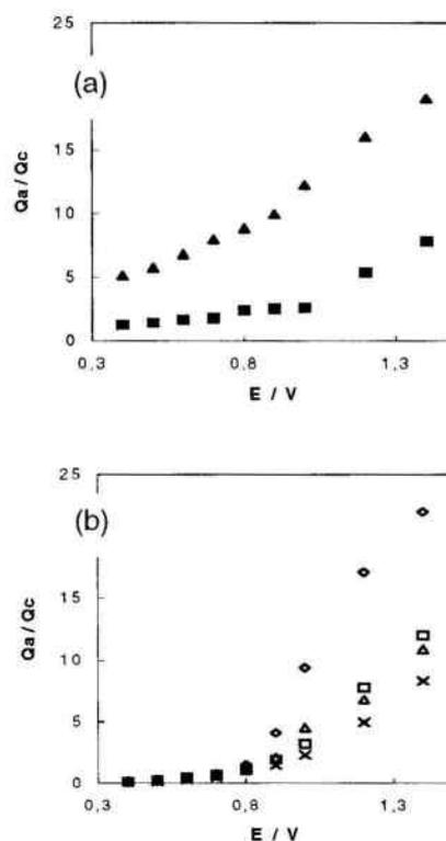
Fig. 4. Dependence of the ratio  $Q_a/Q_c$  on the anodic potential limit: (▲) pyrite alone, (■) pyrrhotite alone and pyrite plus: (◇) 20% pyrrhotite, (□) 40% pyrrhotite, (Δ) 60% pyrrhotite and (x) 80% pyrrhotite.
