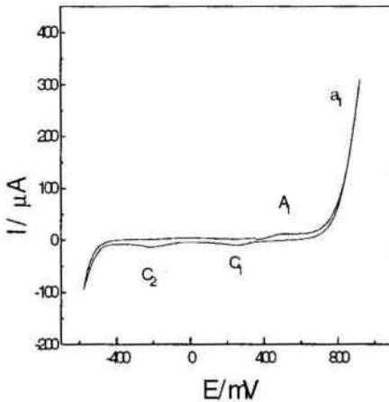
Fig. 1. Voltammogram of pyrite.
