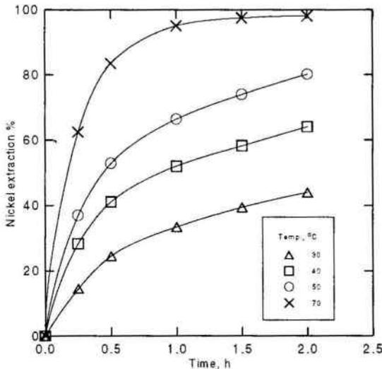
Fig.2. Effect of temperature on nickel extraction (0.5M H<sub>2</sub>SO<sub>4</sub>, 0.2M K<sub>2</sub>Cr<sub>2</sub>O<sub>7</sub>)
