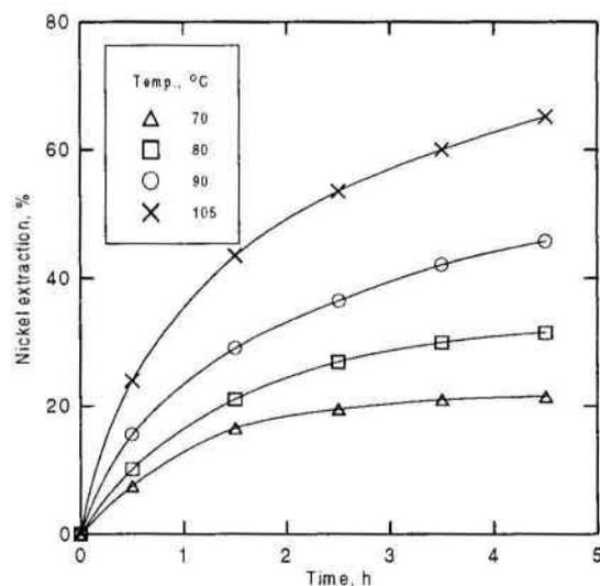
Fig.1. Effect of temperature on nickel extraction (1.5M FeCl<sub>3</sub>, 0.15M CuCl<sub>2</sub>, 3.5M NaCl)
