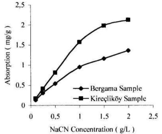
Figure 6. Effect of cyanide concentration on specific absorption.
