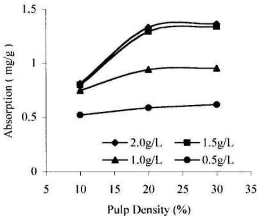
Figure 7. Effect of pulp density on specific absorption behavior of the Bergama sample.
