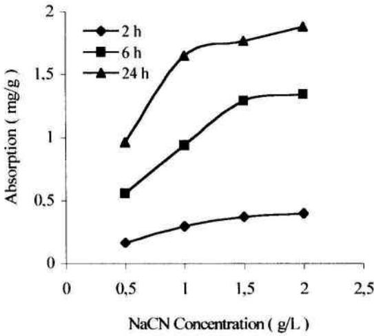
Figure 3. Cyanide concentration versus specific absorption graph of the Bergama sample.
