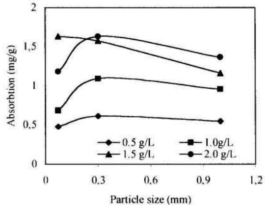
Figure 9. Particle size - specific absorption relationship for the Bergama sample.
