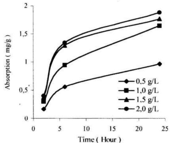
Figure 2. Agitation time versus specific absorption graph of the Bergama sample at different CN<sup>-</sup> concentrations.
