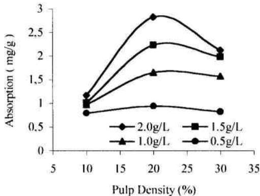
Figure 8. Effect of pulp density on specific absorption behavior of the Kireçliköy sample
