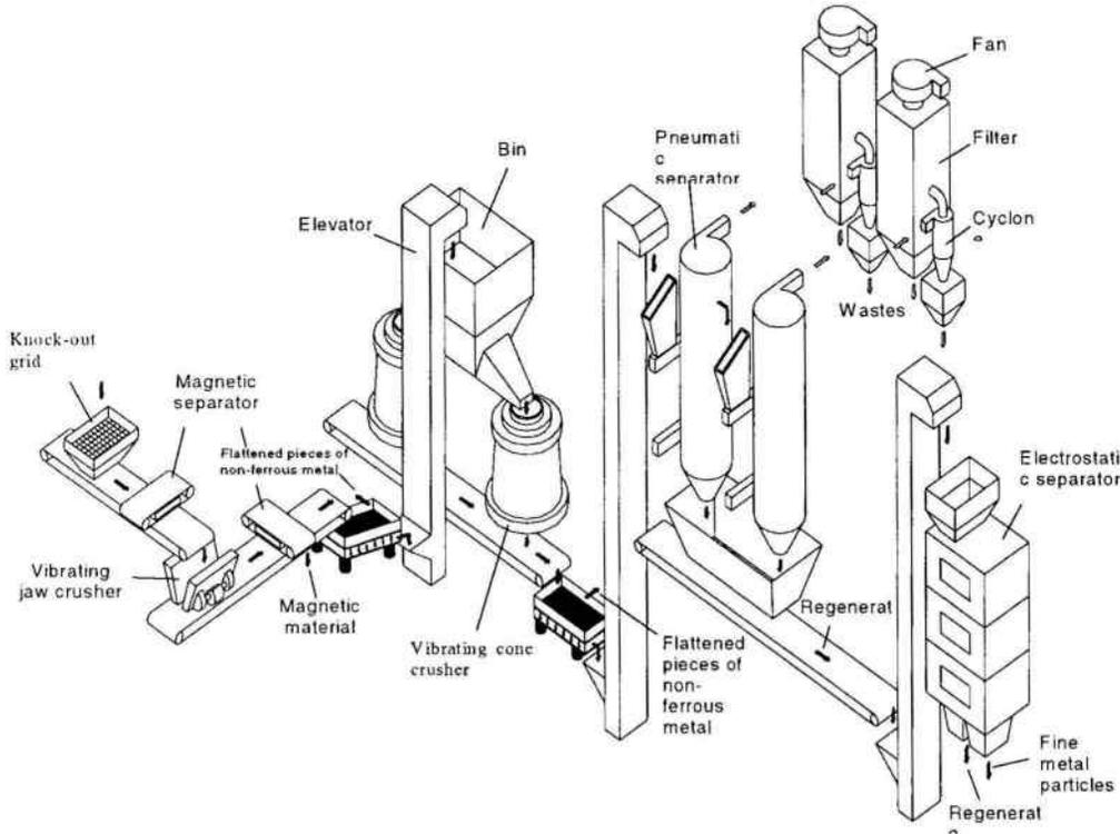
Fig.4. Flowsheet of a line for regenerating casting sands, slags and refractories.
