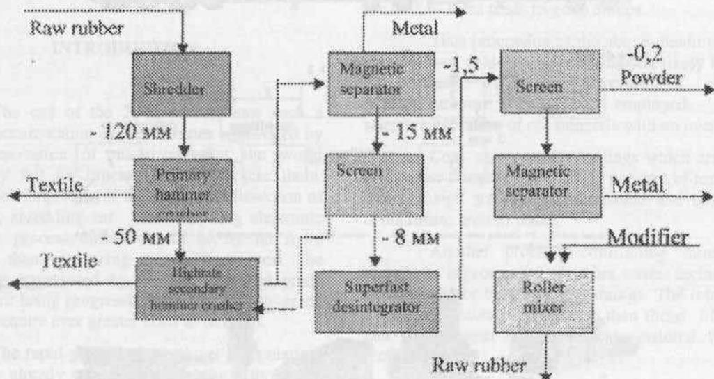
Fig.3 Flowsheet for processing rubber wastes
