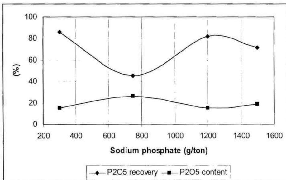
Figure 1 –Metallurgical recovery of  $P_2O_5$  and  $P_2O_3$  concentrate contents at 1200 g/ton of sodium phosphate dosage related to soy bean oil soap dosages at 10.5 pH value.
