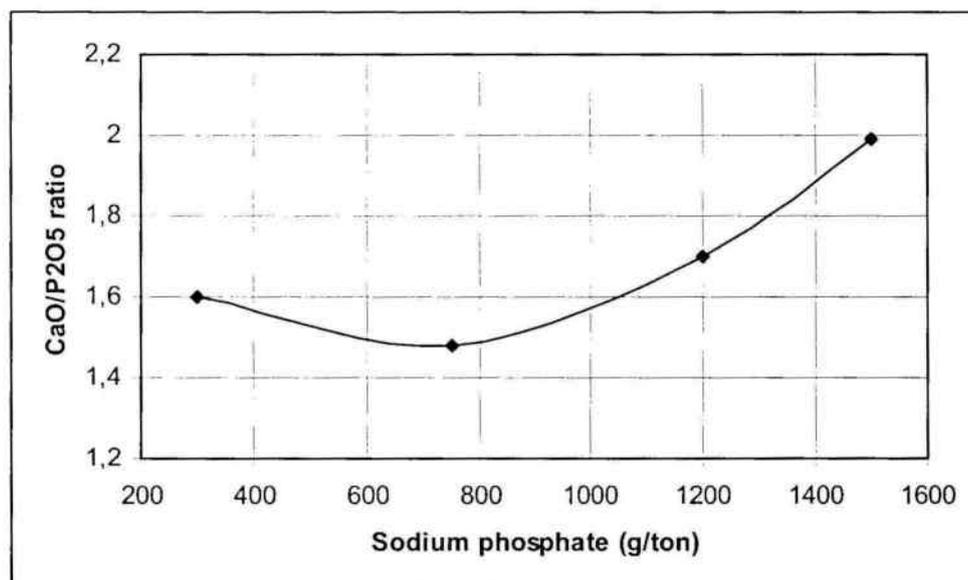
Figure 2 – CaO/P<sub>2</sub>O<sub>5</sub> ratio in the concentrates at 1200 g/ton of sodium phosphate dosage related to the soy bean oil soap dosages at 10.5 pH value.
