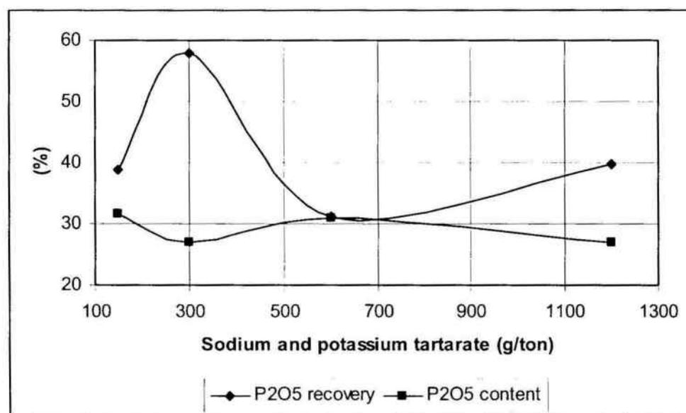
Figure 3 – Metallurgical recovery of P<sub>2</sub>O<sub>5</sub> and P<sub>2</sub>O<sub>5</sub> concentrate contents at 300g/ton of soy bean oil soap related to sodium and potassium tartarate dosages at 10.5 pH value.
