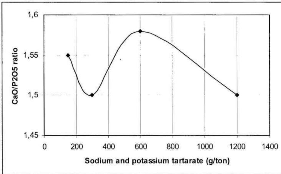
Figure 4 – CaO/ $P_2O_5$  ratio of the concentrate at 300 g/ton of soy bean oil soap dosage related to sodium and potassium tartarate dosage at 10.5 pH value.
