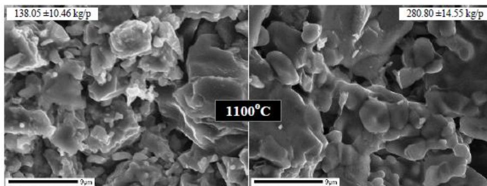
**Figure 2. Microstructures of pellets; bentonite bonded at left, calcined colemanite bonded at right.**
