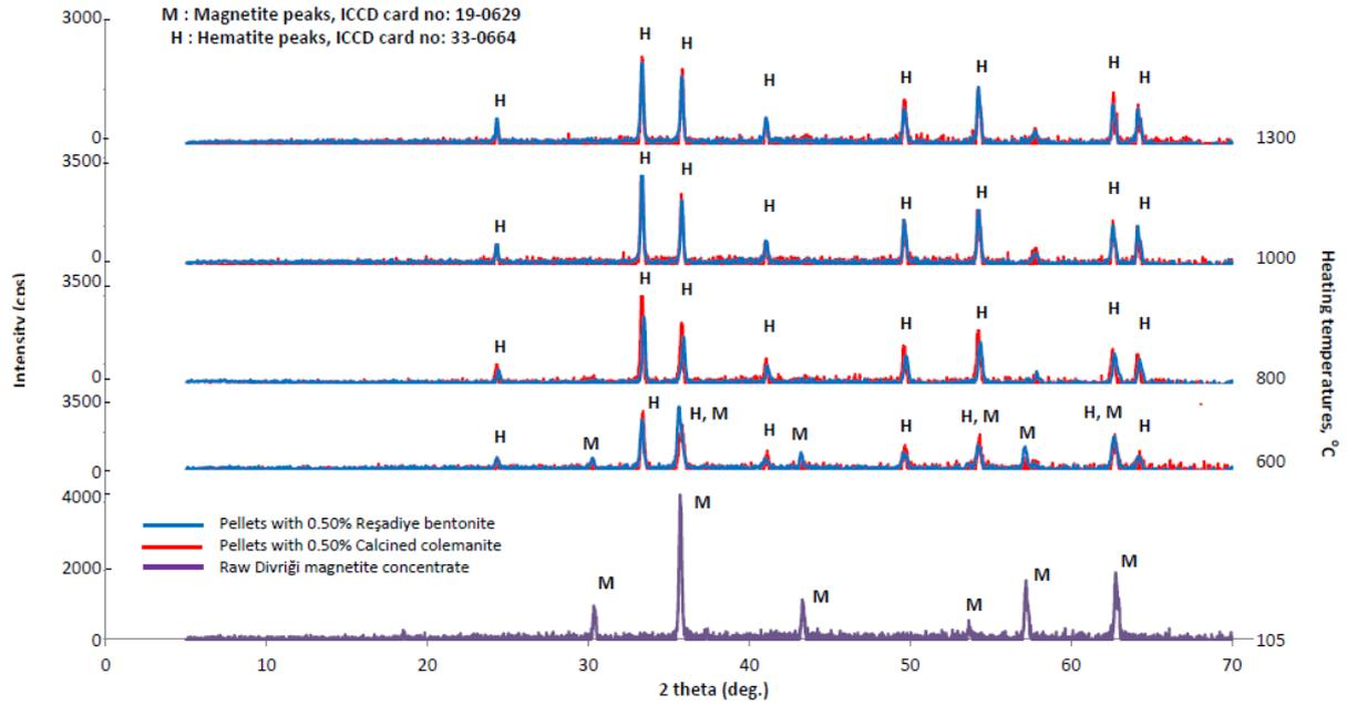
**Figure 3.** X-ray diffraction patterns of dry magnetite concentrate (purple) and pellets made from this concentrate and produced with 0.50% bentonite (red) or 0.50% calcined colemanite (blue) and heated at 600-800-1000-1300°C for 30 minutes.
