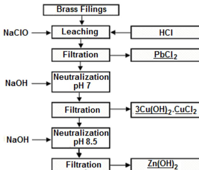
Figure 3. Process and unit operations for extracting copper and zinc from brass filings.
