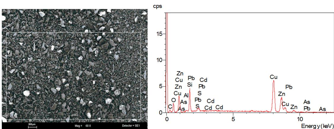
Figure 2. The SEM micrograph of a brass filings sample and corresponding EDS spectrum.
