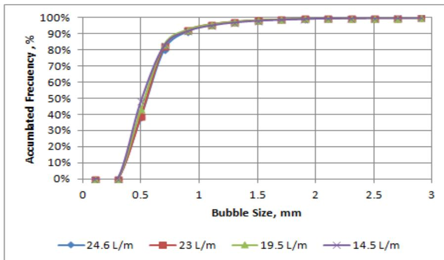
Figure 6. Cumulative distribution of bubble size in self-aerated cell, at different air flux. Assays at 4,121 mosl.
