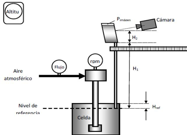
Figure 3. Schematic disposal of measurement system.
