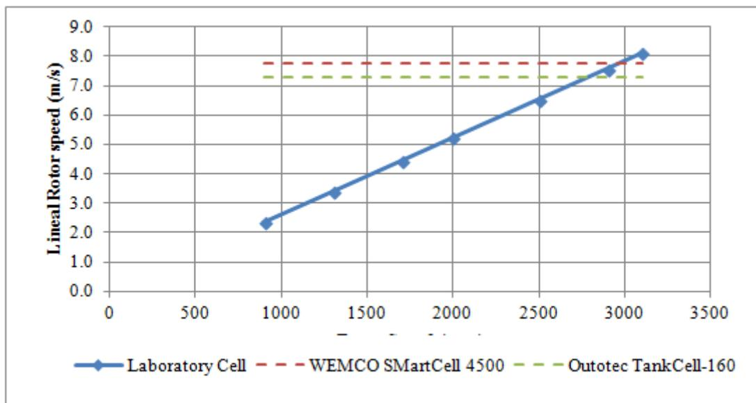
Figure 2. Lineal rotor speed in a laboratory and industrial Cells.
