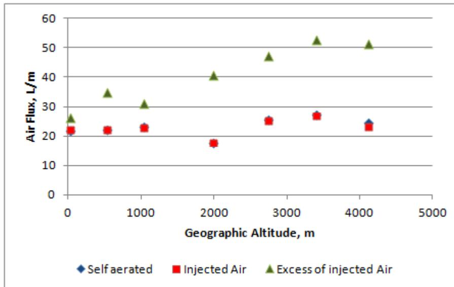
Figure 9. Air flux on self-aerated cell and injected air cell in different geographic altitudes.
