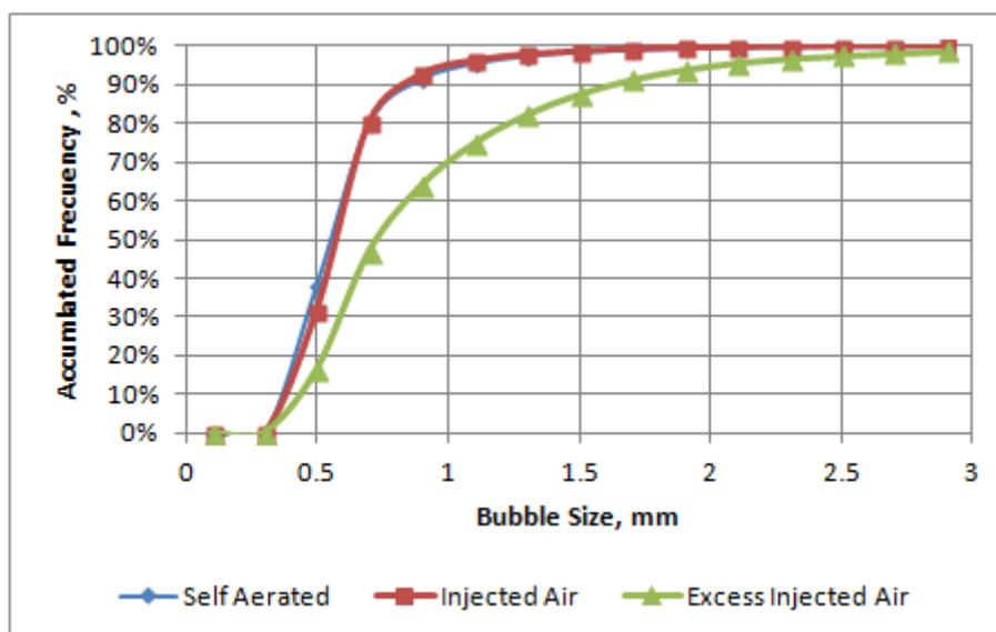
Figure 11. Cumulative distribution of bubble size with with self-aerated and injected-air cell.
