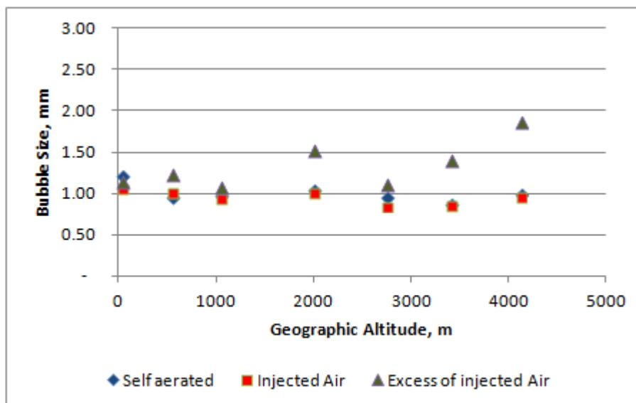
Figure 10. Effect of geographic altitude on bubble size with self-aerated and injected-air cell.
