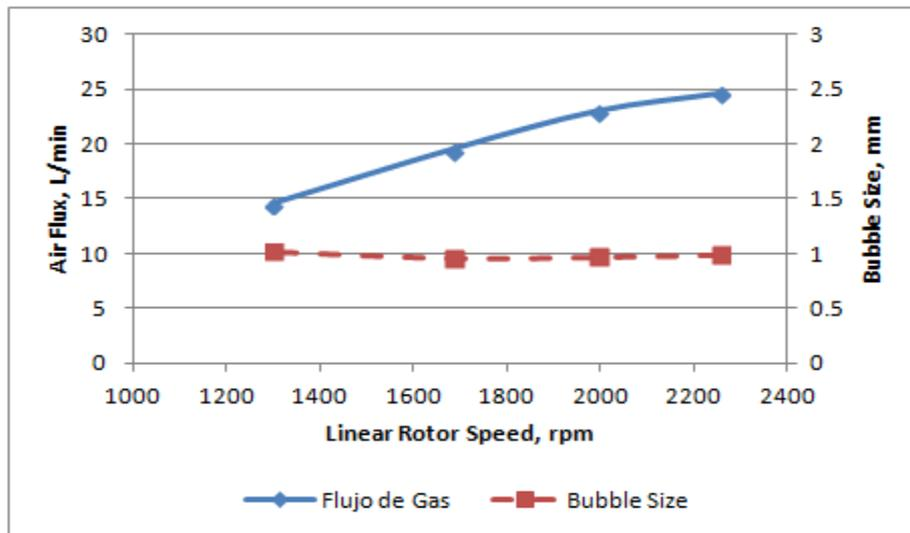
Figure 5. Effect of lineal rotor speed on air flux and bubble size.
