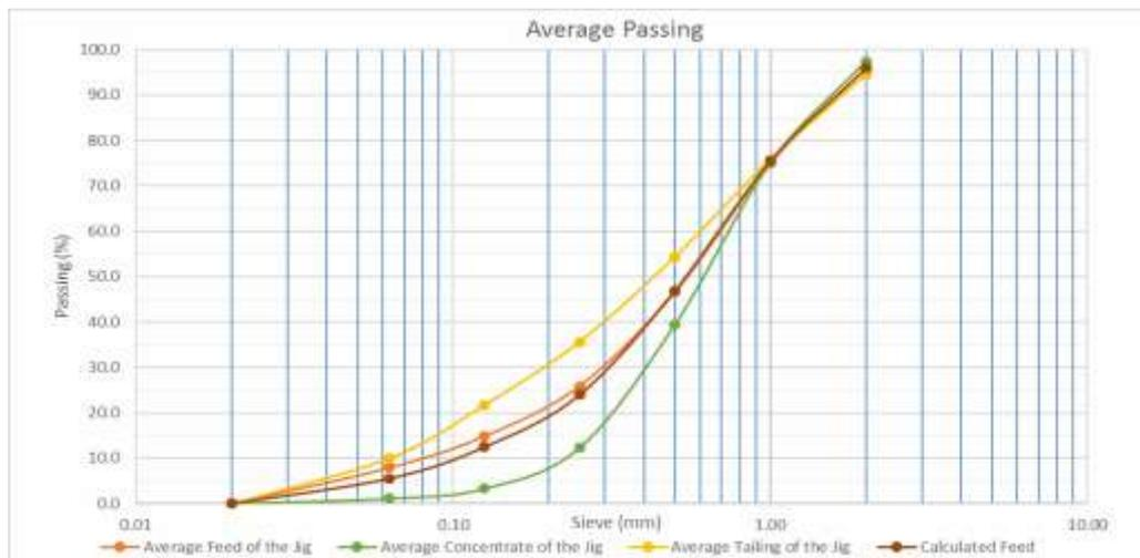
Graph 2. A graphical view of the average passing results of the PSD of test 2.
