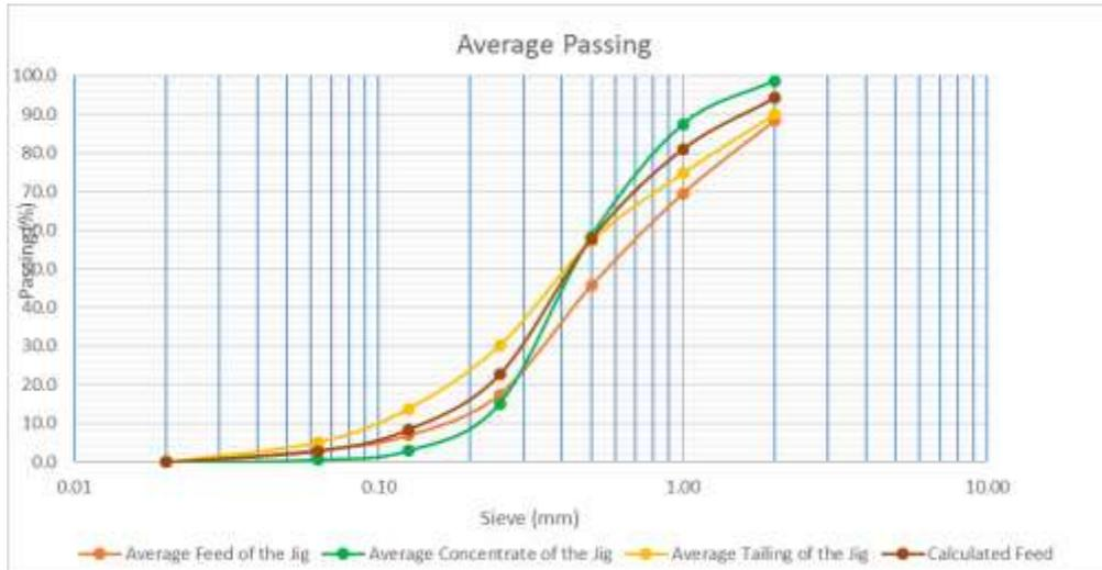
Graph 1. A graphical view of the average passing results of the PSD of test 1.
