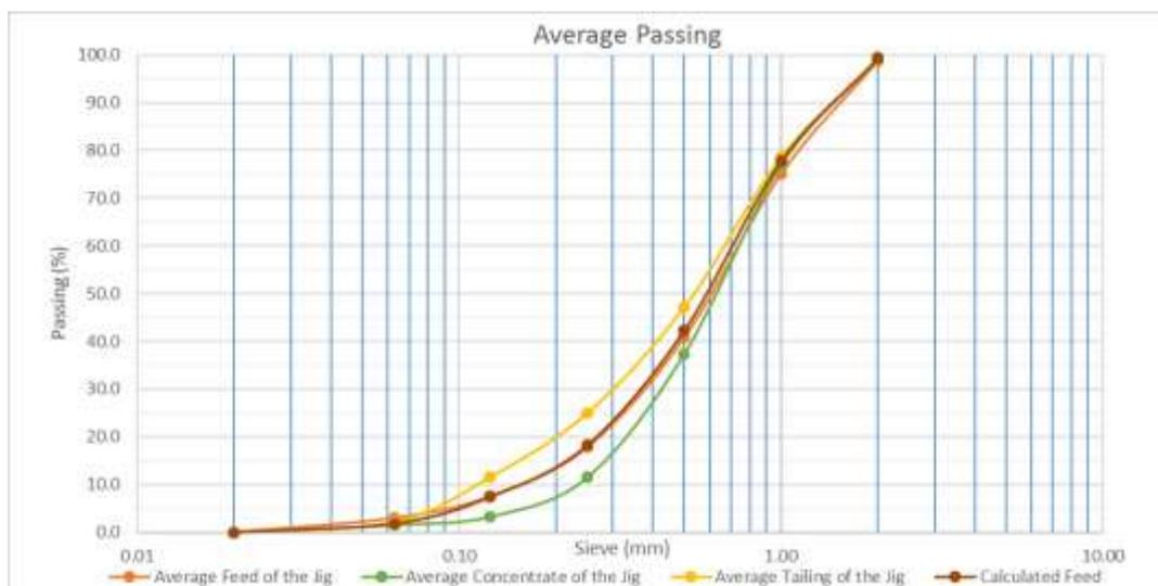
Graph 3. A graphical view of the average passing results of the PSD of test 3.
