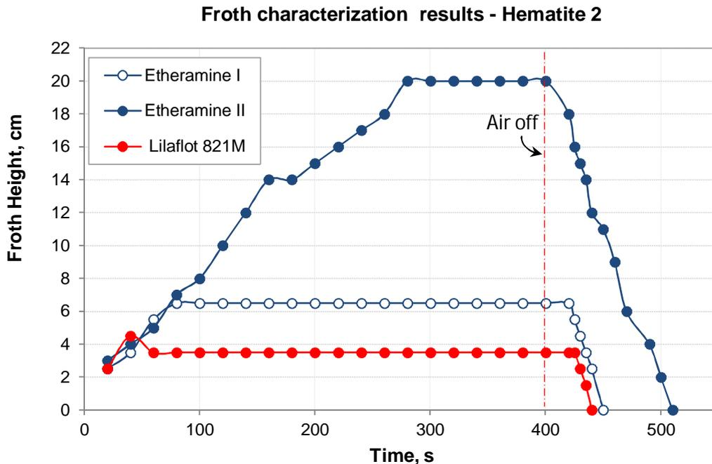
Figure 4. Frothing profiles for different etheramines.
