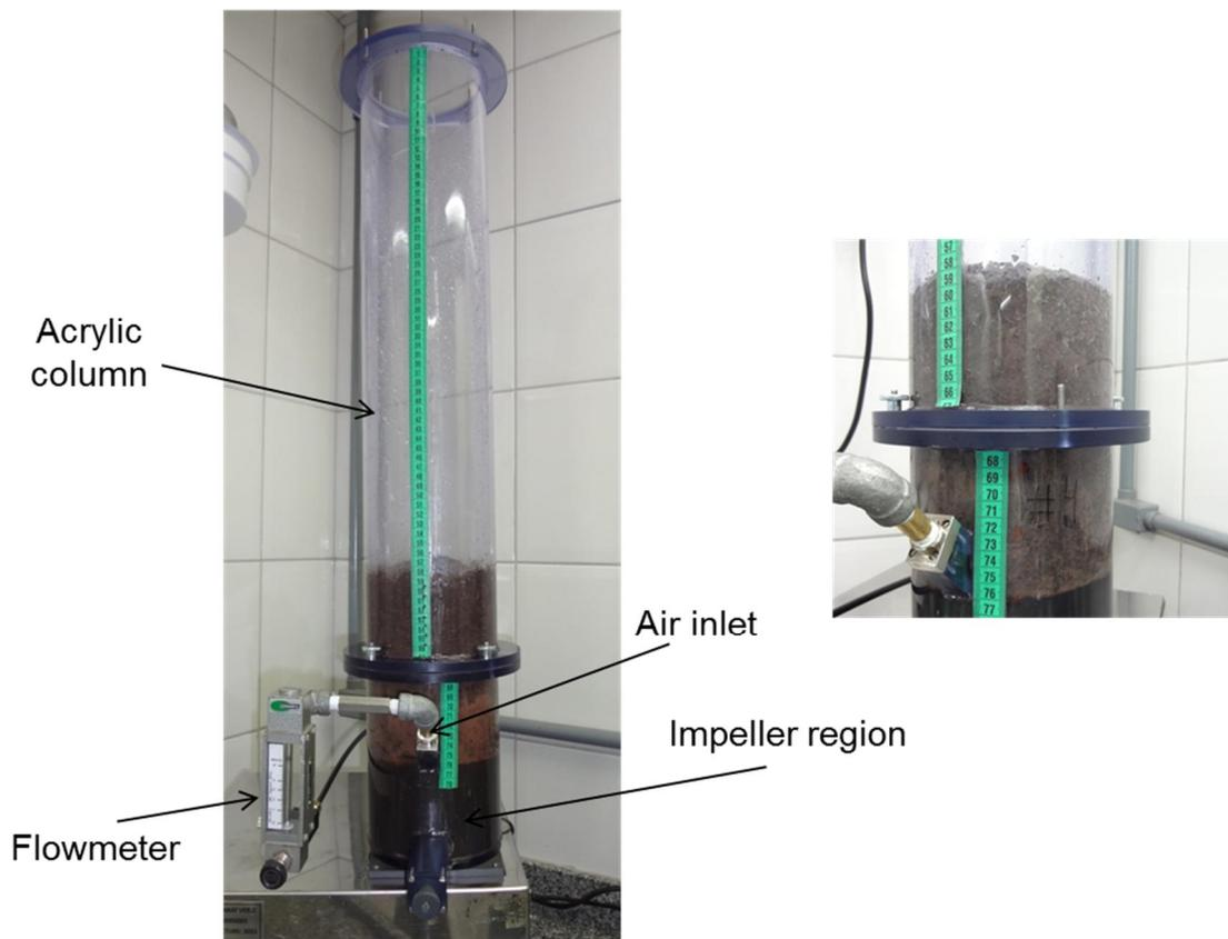
Figure 2. Frothing machine. Detail of a frothing test.
