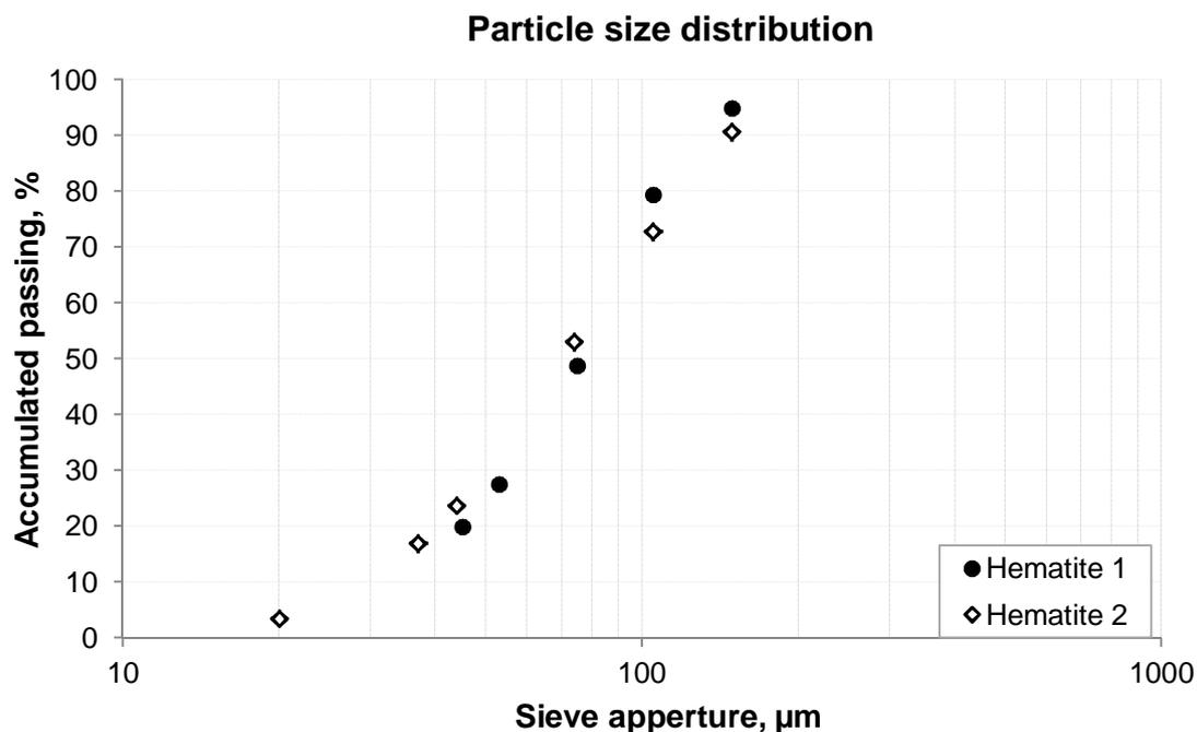
**Figure 1. Particle size distribution – Hematite 1 and Hematite 2.**
