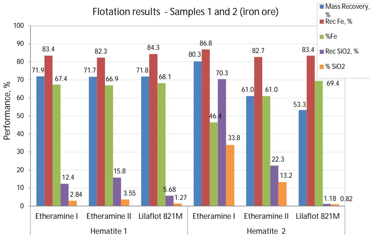
Figure 3. Comparative flotation results using Lilafлот 821M and conventional etheramines based collectors.
