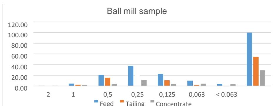
Figure 9. Histogram showing the retained material of the ball mill sample
