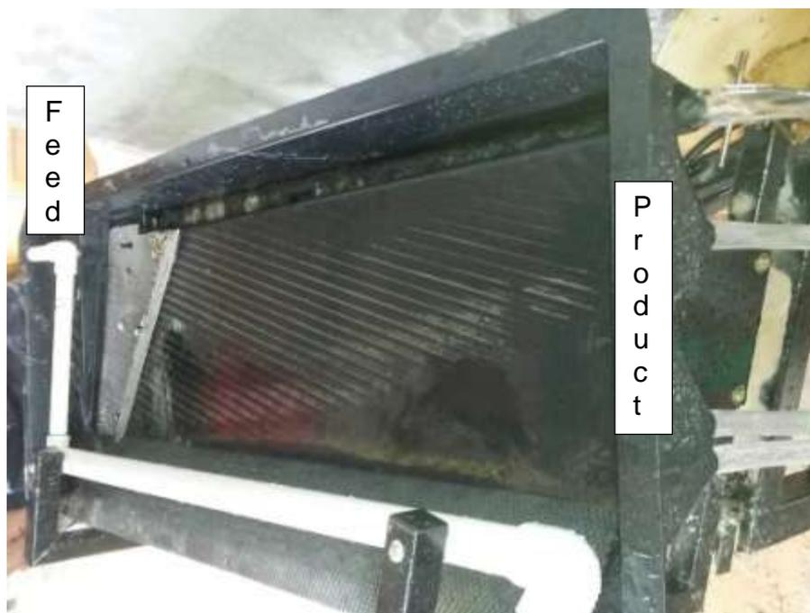
Figure 1. Photograph showing the deck of the Rp4 shaking table
