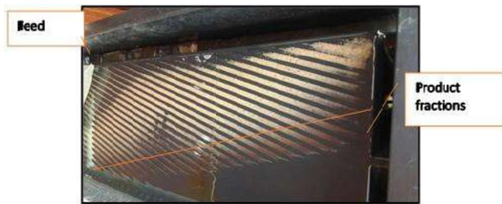
Figure 2. Photograph showing the division between the light and heavy materials
