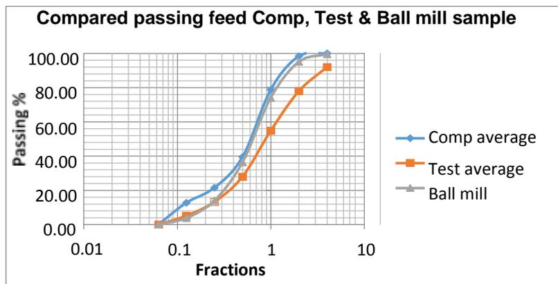
Figure 4. Graph showing the compared passing of the feeds
