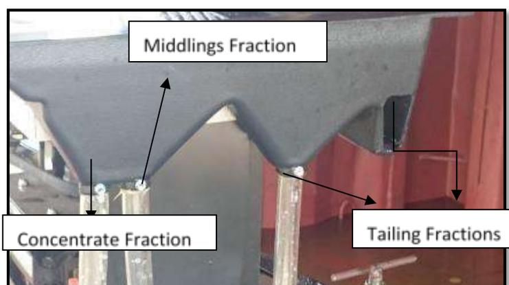
Figure 3. Product fractions of the Rp4 shaking table
