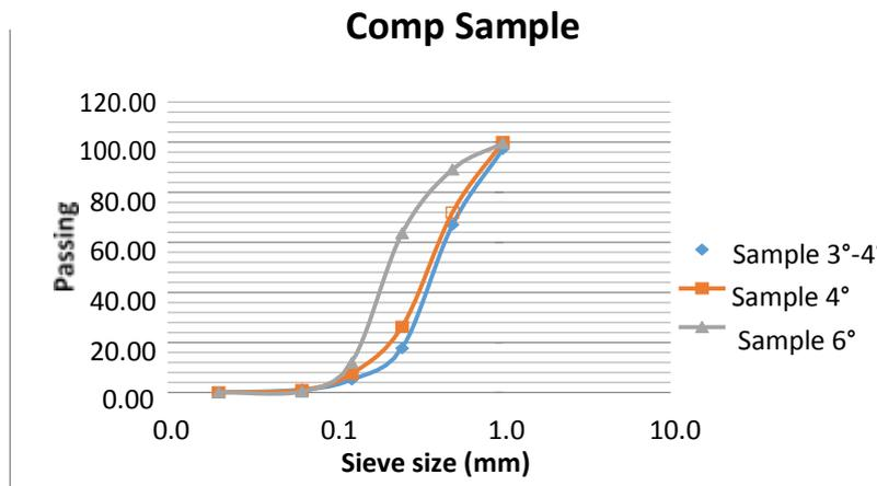
Figure 5. Graph showing the tailing passings of the composed sample
