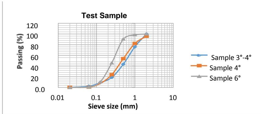
Figure 7. Graph showing the passing of tailing test sample
